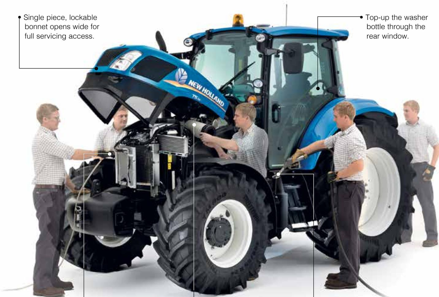
• The cooling package slides out for simple and efficient cleaning.
