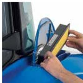
Replace or clean the cab air filter by simply removing from the easy access fender-mounted position.
